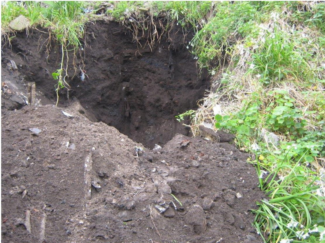
Plate 6 – Ash Core Identified in TP106
