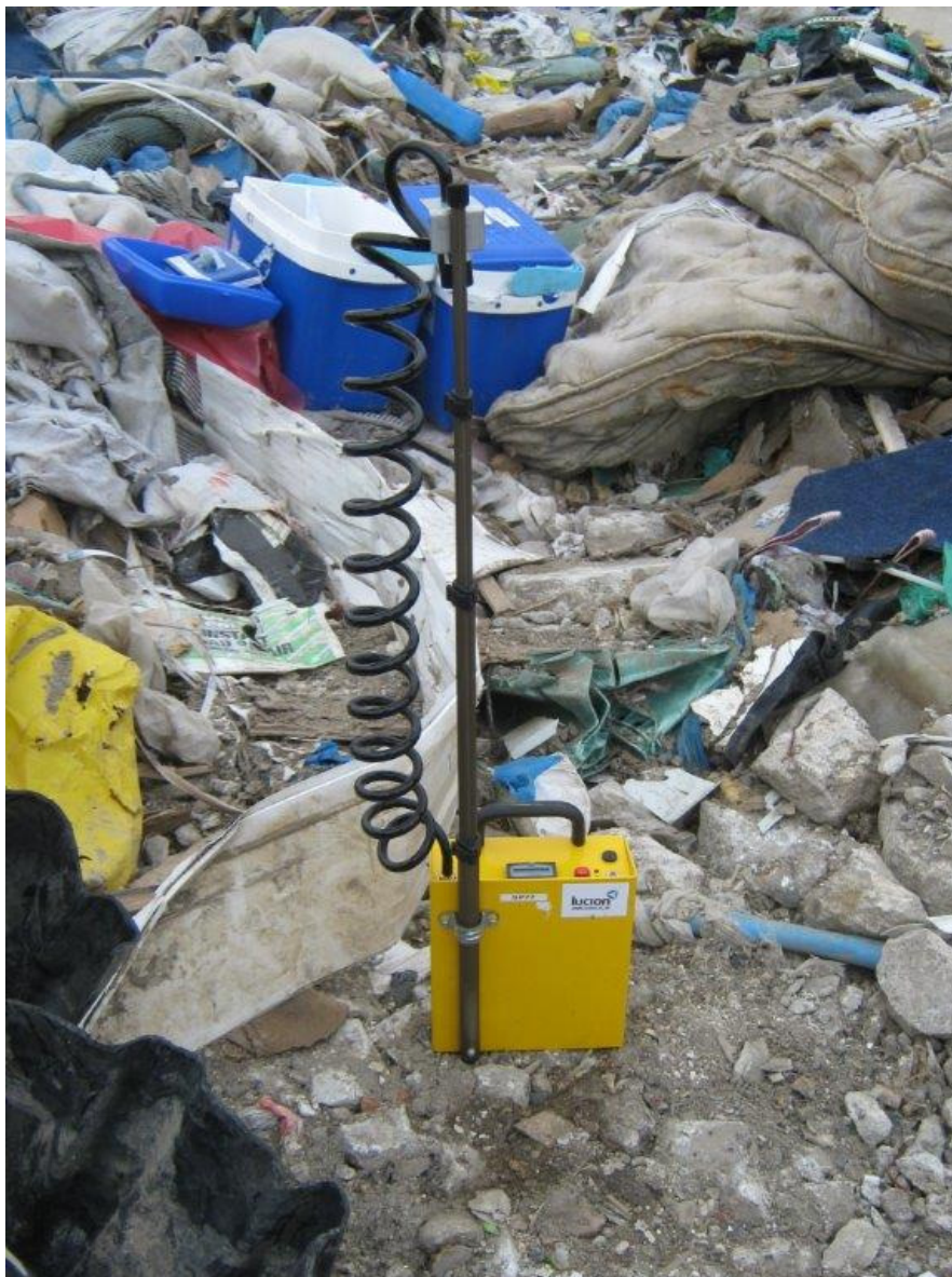
Plate 21 – Asbestos Air Monitoring Pump
