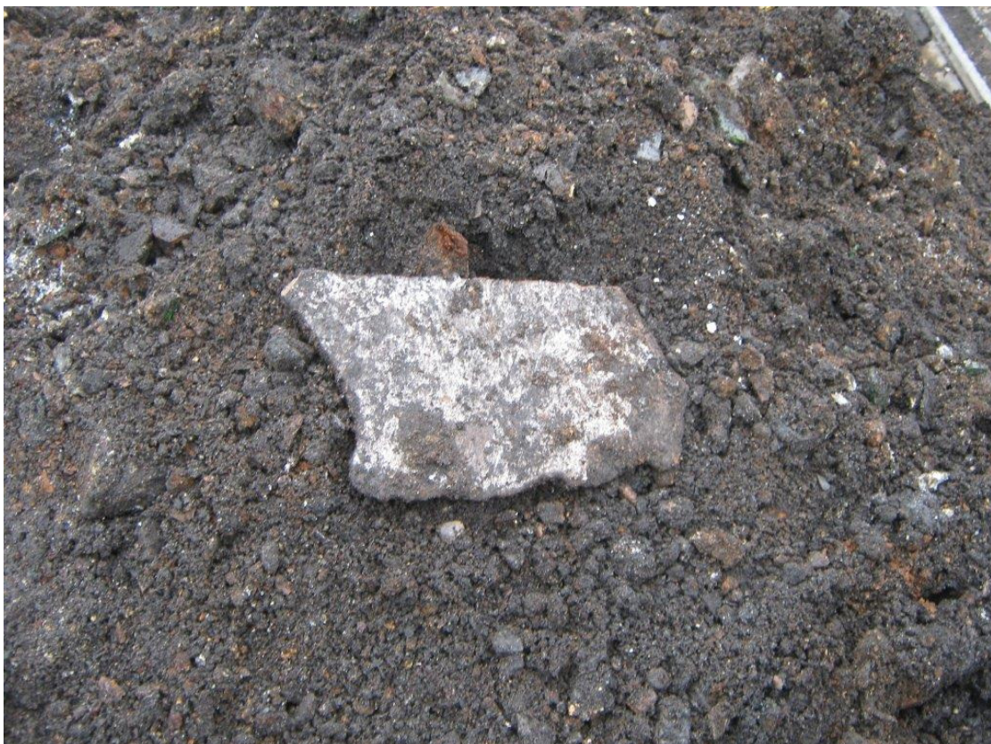
Plate 3 – Suspected Asbestos Fragment within IBA
