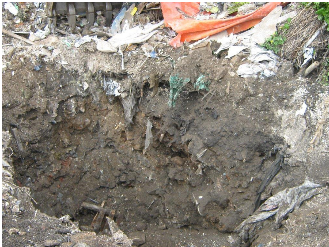
Plate 11 – Asbestos Pocket in TP110
