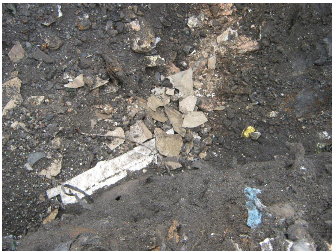
Plate 11 – Asbestos Pocket in TP110
